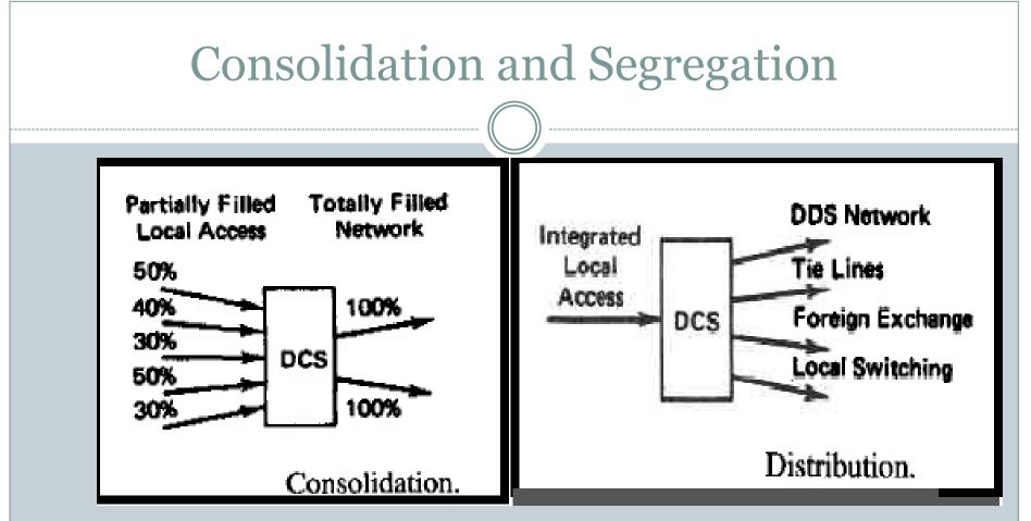
Two basically different DCS grooming functions are depicted in Figures are consolidation and segregation. When multiple-access lines carrying traffic destined to a common distant node are partially filled, the per-channel costs of transport to the remote node can be reduced by consolidating the traffic. Conversely, when different types of traffic originate at a single location, it is desirable to allow a single facility to carry all types of traffic and segregate it at the DCS.
